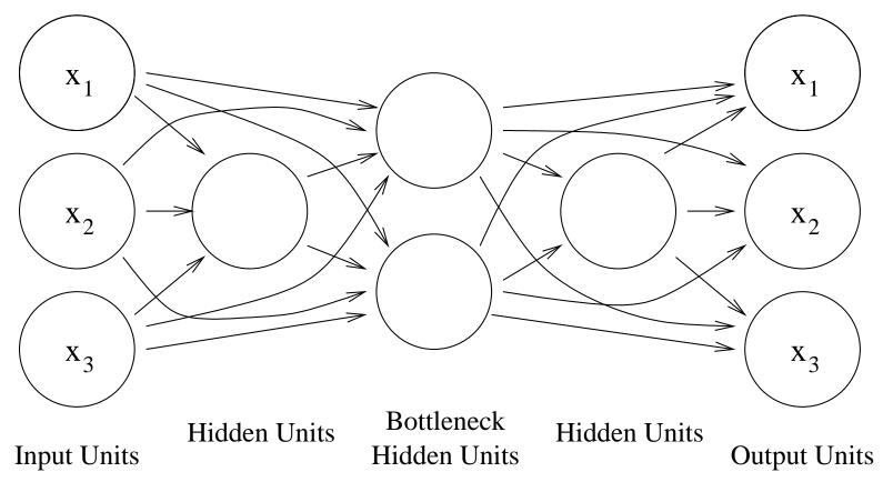
Here, I've put in direct connections from the inputs to the middle hidden layer (the bottleneck) and from the bottleneck to the output units. I show only one hidden unit in the extra hidden layers, but usually there would be more.
